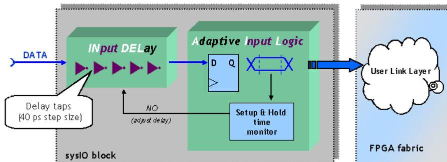
The key to this mode is the fact it is a self-contained, closed loop system that can be enabled/disabled under FPGA control. The closed loop design also allows for tracking and compensating for delay variations due to process, voltage and temperature conditions.
