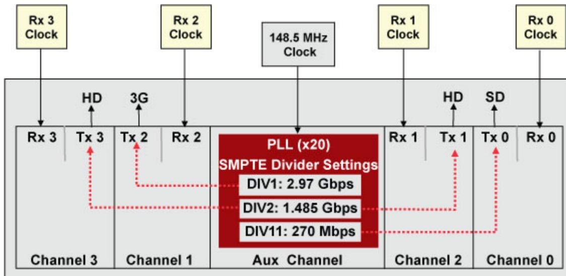
**Figure 6 - Enhanced SMPTE Multi-rate Support in the LatticeECP3 SERDES**
