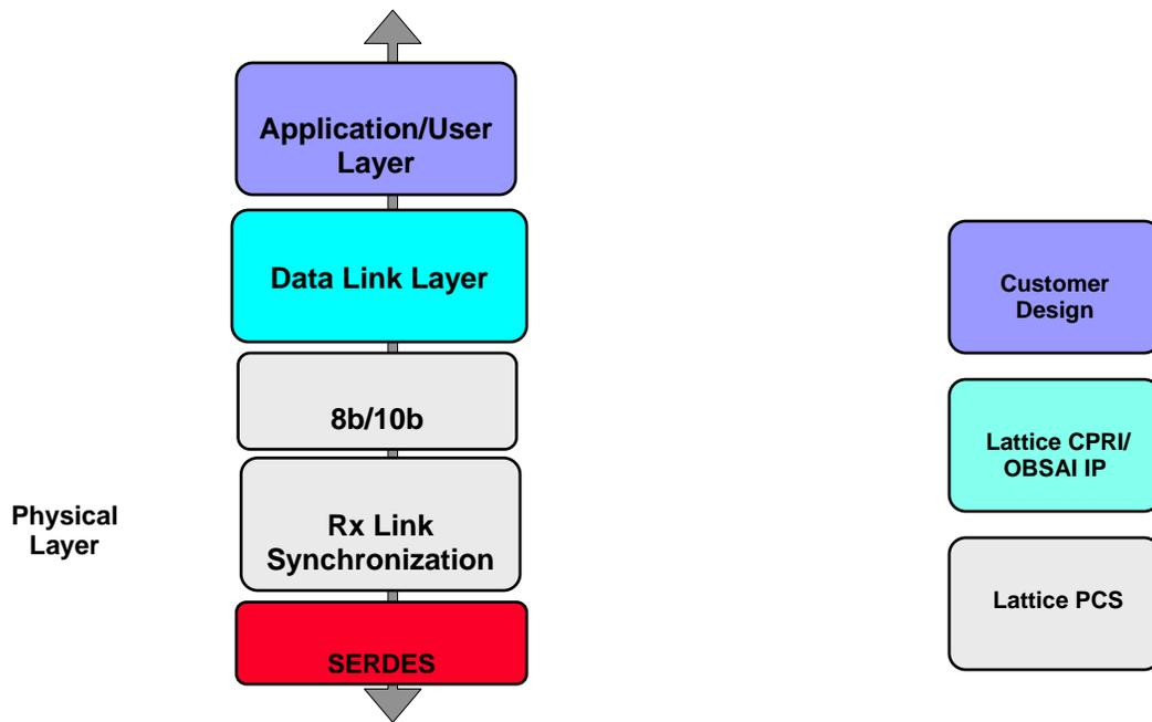
**Figure 4 - CPRI/OBSAI Protocol Stack Supported by the LatticeECP3**
