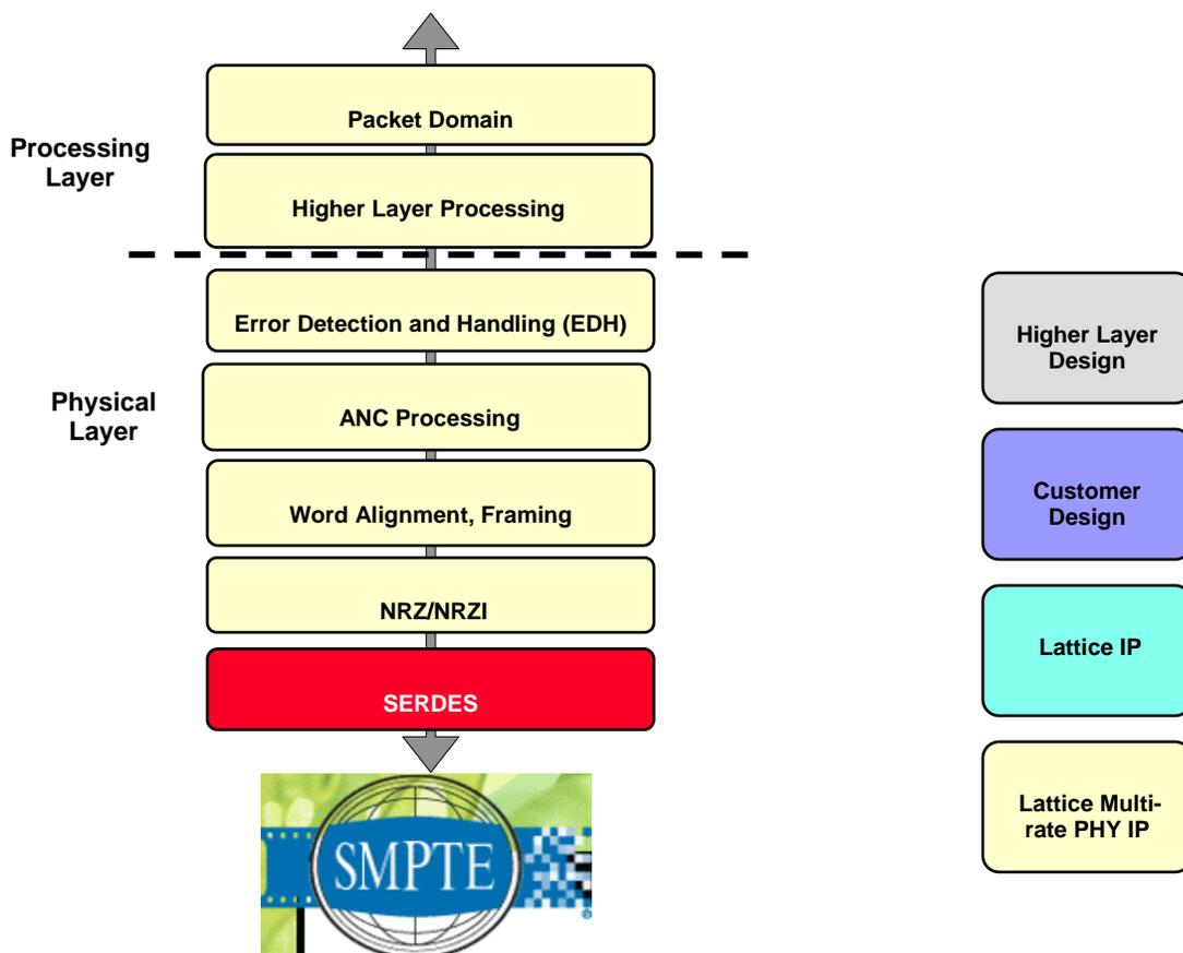
**Figure 7: SMPTE Protocol Stack Supported by the LatticeECP3**
