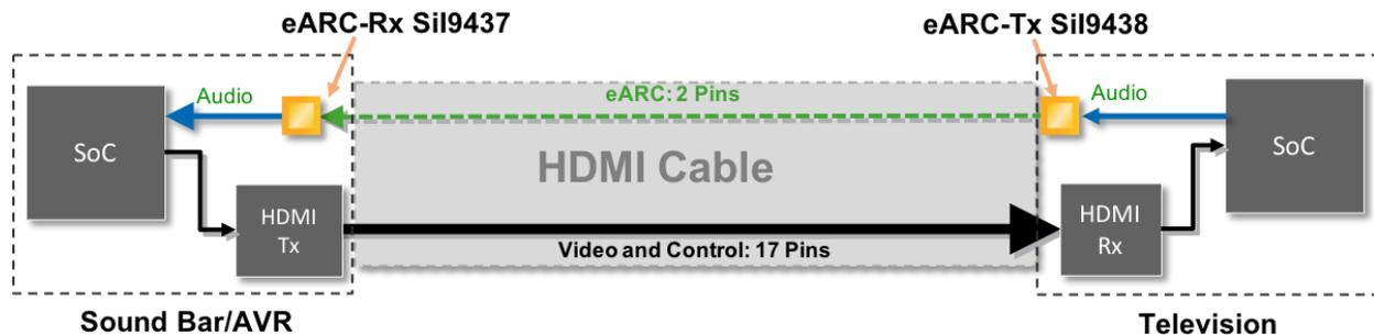
**Figure 3: Lattice Sil9437 and Sil9438 Solutions for eARC**
