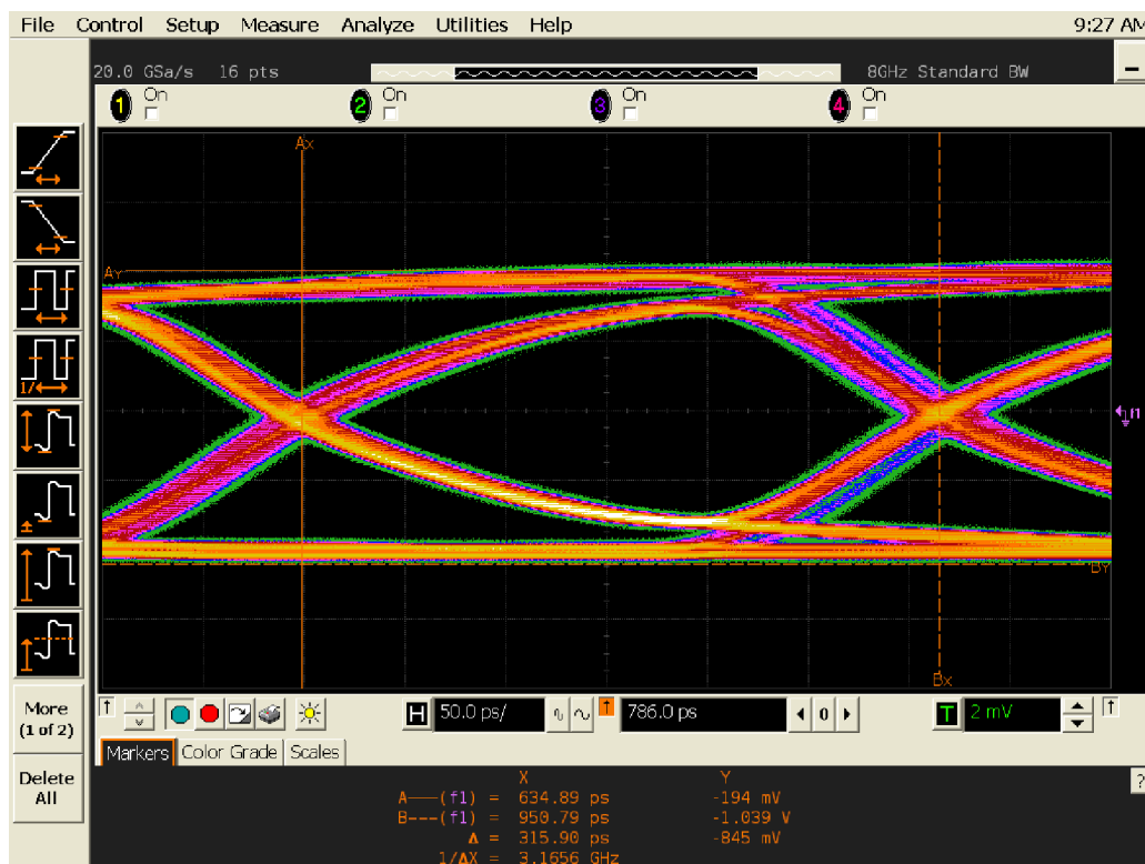
Figure 9. DSO Differential Eye Diagram with PCS Quad PCSB and No Backplane
