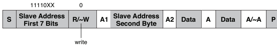
Figure 6. Master Write Operation for 10-Bit Addressing
