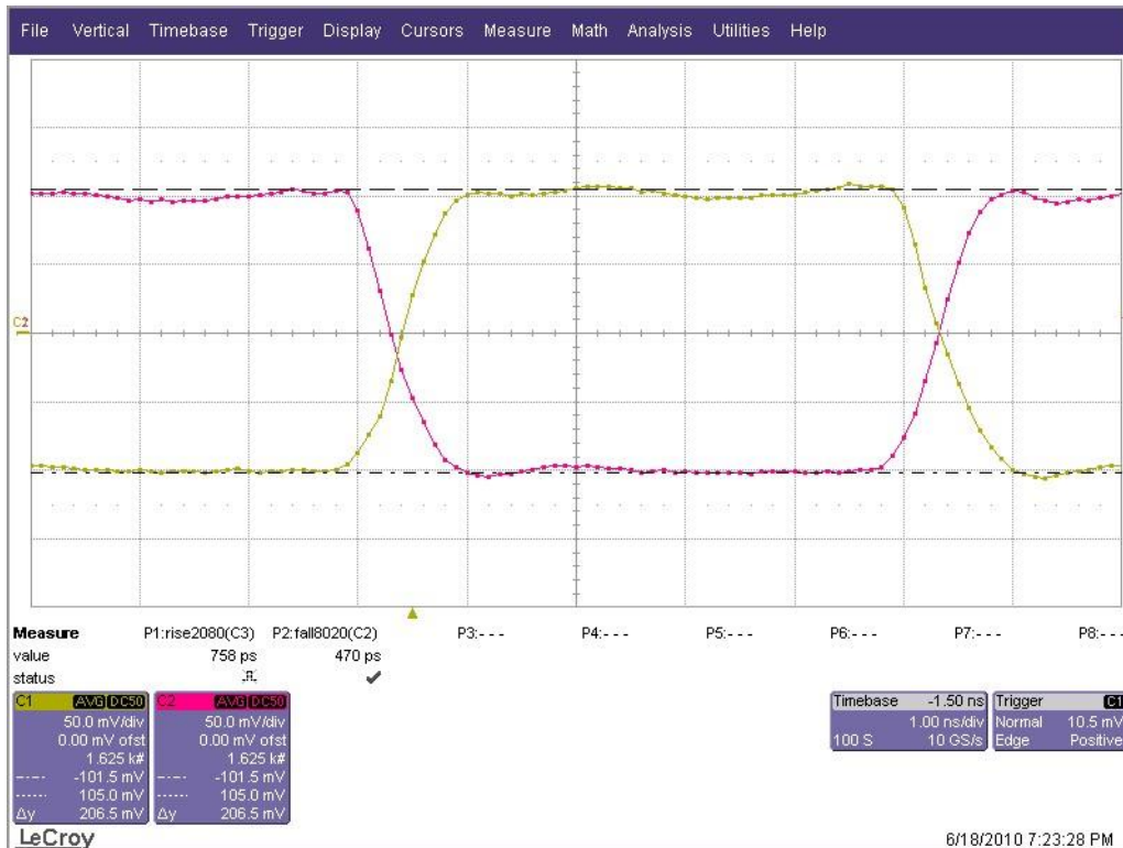
Figure 2.4. Typical Differential Output Waveform from Hardware Test
