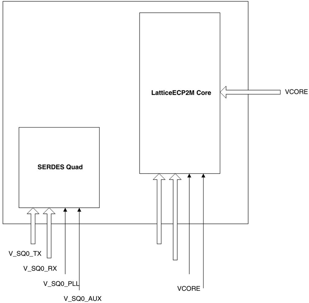
The SERDES quad in the LatticeECP2M-35 has power supply voltages isolated from the LatticeECP2M core logic supply. If a LatticeECP2M-50 is placed onto a circuit board originally designed for a LatticeECP2M-35, the new SERDES quad will be powered by the same supply voltage as the core logic. This is permissible as long as the new SERDES quad is not used. The new SERDES quad can be seen in Figure 2.
