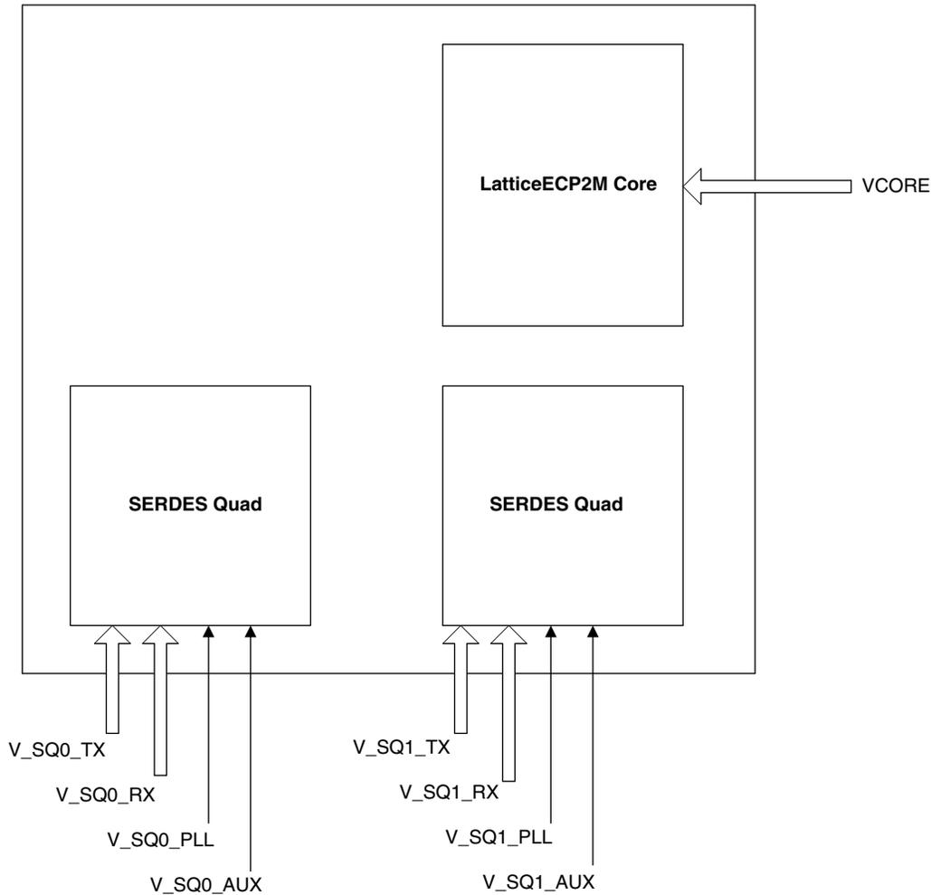
As can be seen in the diagram above, the SERDES quads have independent supply inputs. The natural desire for a design implemented with the LatticeECP2M-50 is to connect the quiet and isolated SERDES power supply to both the SERDES quads. This is convenient from the point of view of creating an isolated and quiet supply plane for the circuit board. This technique is permissible as long as the LatticeECP2M-50 is the only device to reside on the PCB.
